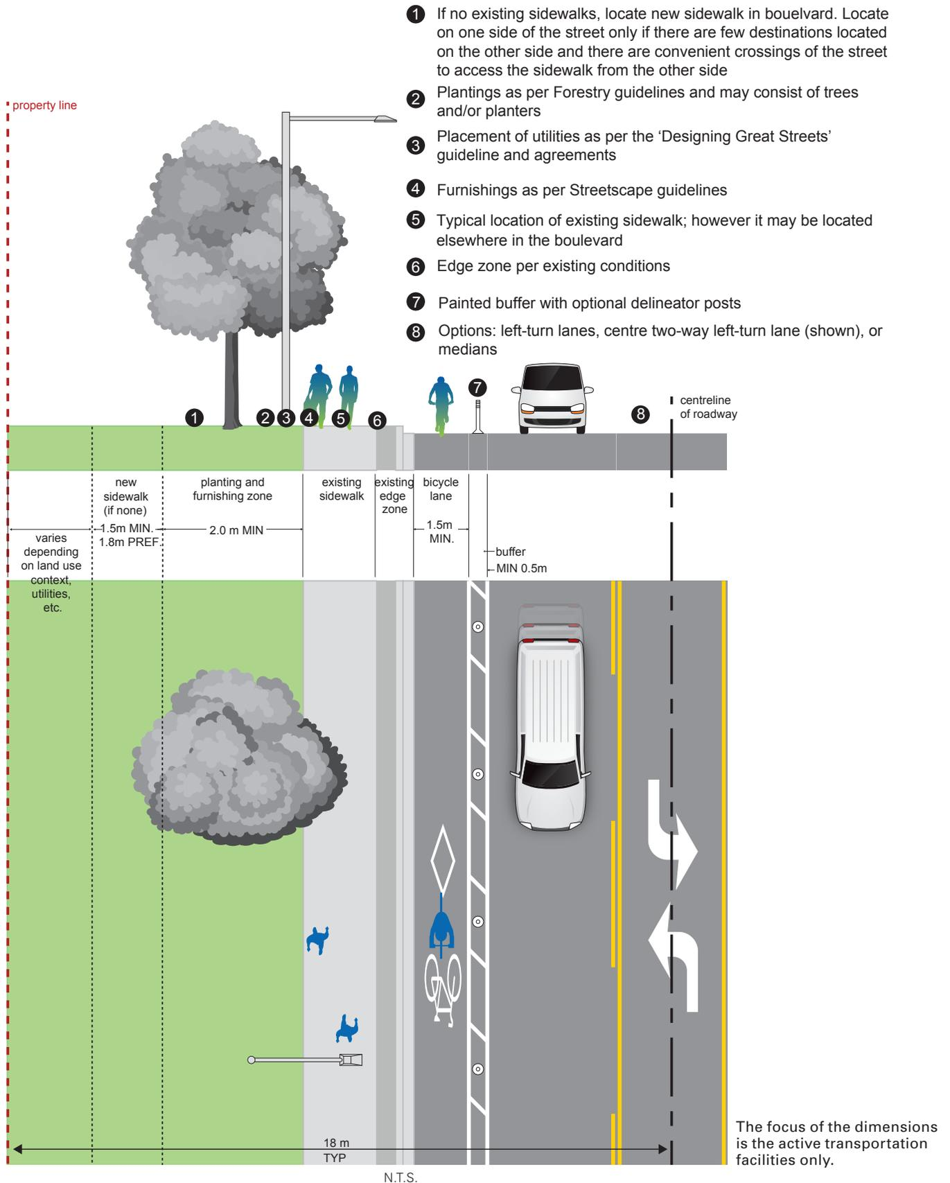
Exhibit 4-31. Retrofit (36 m ROW) - Multi-use path constructed on one or both sides of the street in the boulevard
