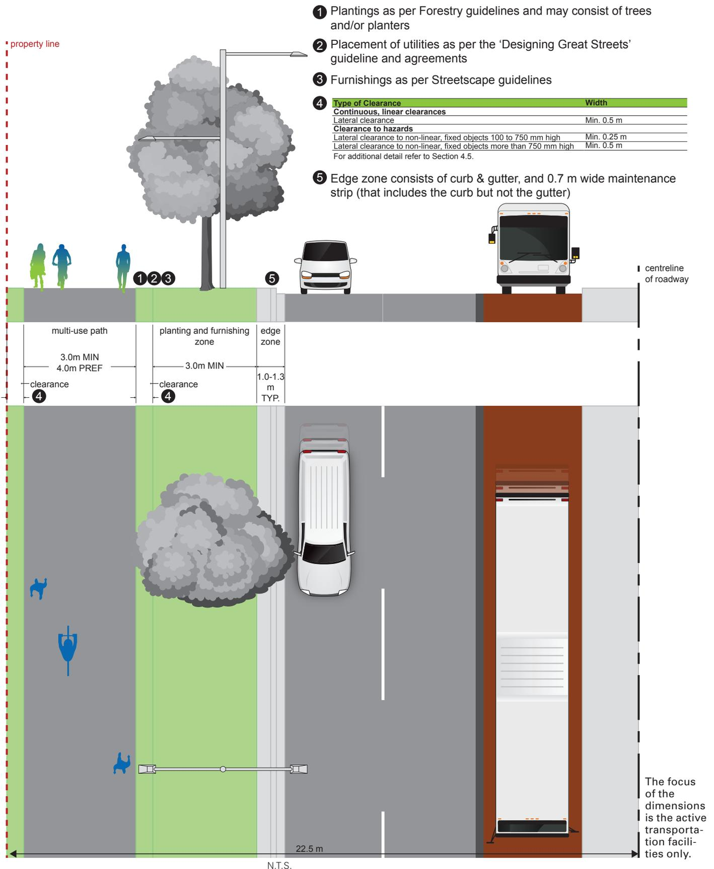
Exhibit 4-22. Connector (45 m ROW) - Sidewalks and in-boulevard cycle tracks with four travel lanes and rapid transit
